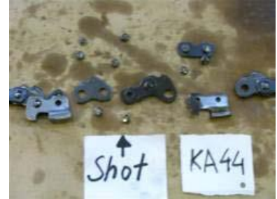
Linkages from a failed chain
