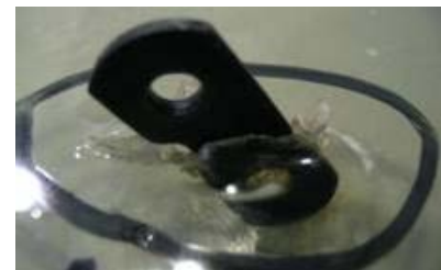
Chainlink embedded in a cab window
