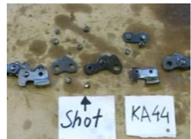
Linkages from a failed chain
