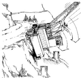
Because of the enormous tension heavy loads place on the yarder, tree's and anchors; cable yarding failures are very dangerous. When a tailhold tree or stump fails it can destabilize the yarder. Yarders can weigh up to 120 tonnes and may seem incredibly steady but the forces applied when pulling a turn of logs, tensioning guylines or operating from an unstable surface can easily topple this equipment.
