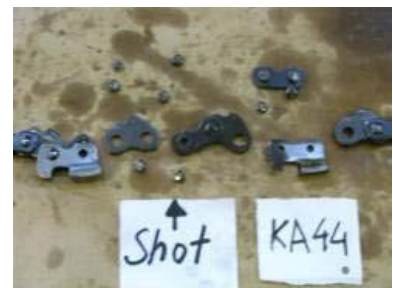
Linkages from a failed chain
